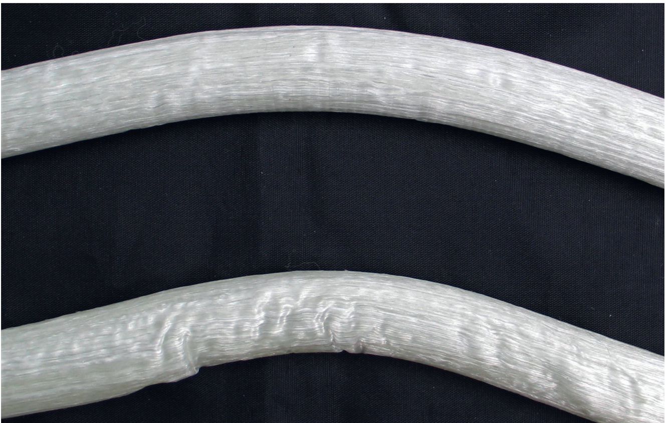
Comparison of fiber wrinkling on a test specimen produced by local stretch bending (above) and a test specimen produced by draw bending (below)
