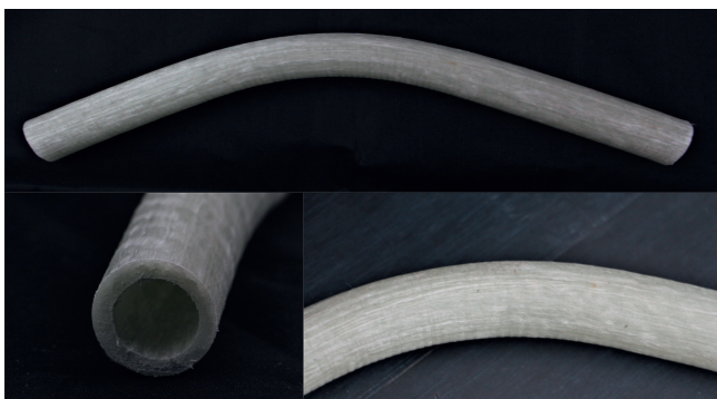
Fig. 2. Hollow profile formed by local stretch bending
